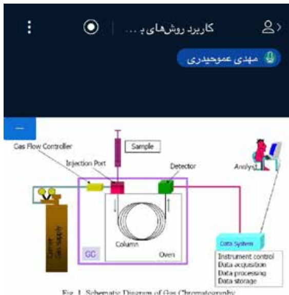
Fig. 1. Schematic Diagram of Gas Chromatography
